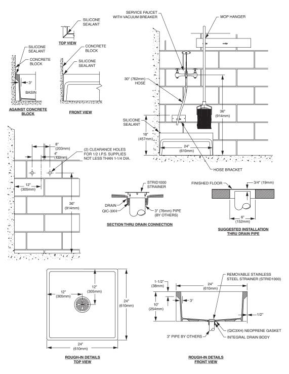
**Installation Note :** QIC32 Quick Drain Connector for 2" pipe or QIC3SN Quick Drain Connector for cast iron soil pipe must be ordered separately.
